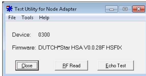
The first thing we must do is to make sure the receiver works properly. Click on the **RF Read** button, and you'll see a screen similar to this:
